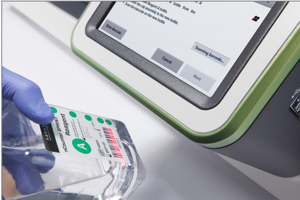
FIGURE 7.7 Scan the bottle using the barcode reader under the instrument touchscreen.
