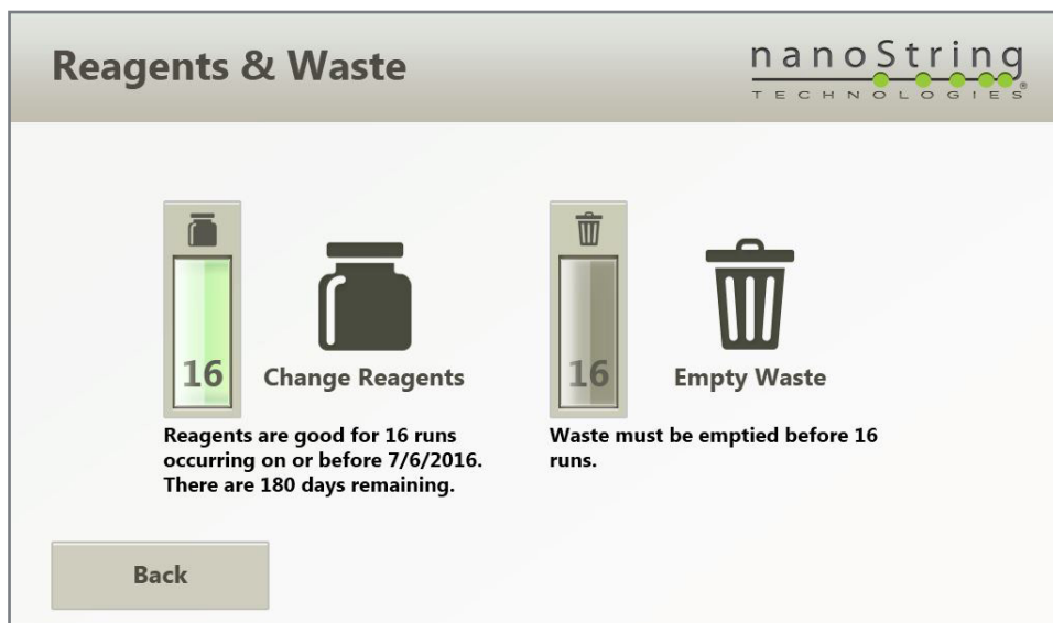
FIGURE 7.4 The Reagents & Waste screen when reagents are full and waste is empty.
