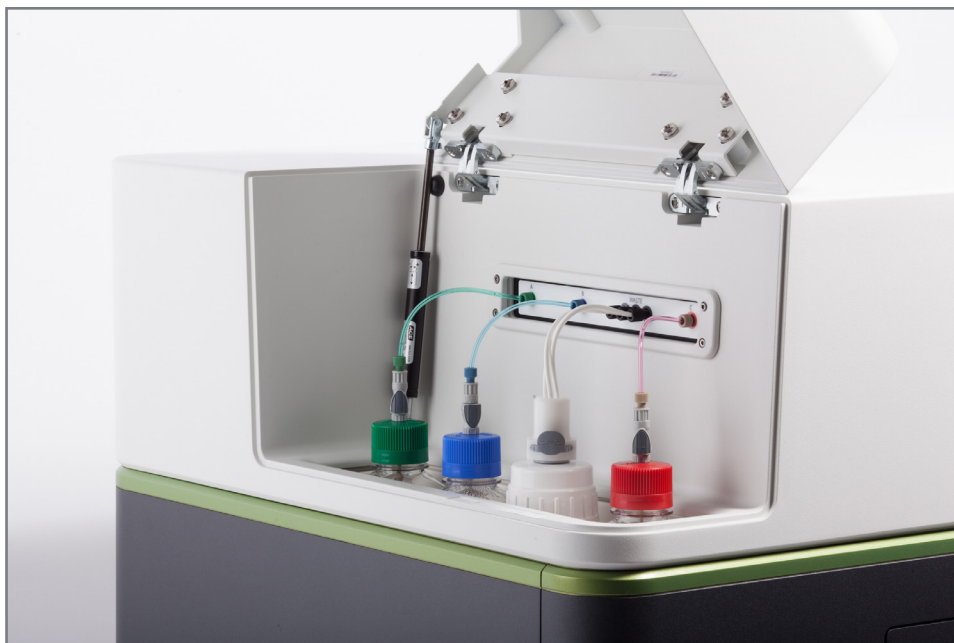
FIGURE 7.2 The reagent bottles and waste bottle inside their compartment. Bottle labels should face the front of the instrument (not the side).
