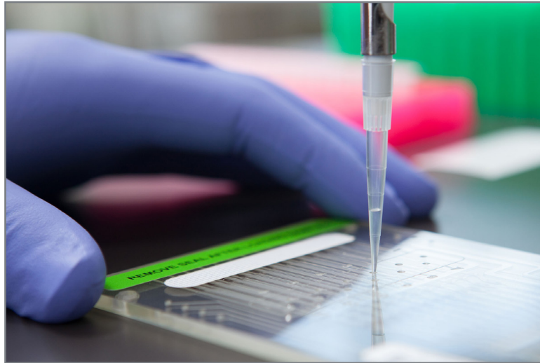
FIGURE 5.3 Demonstration of proper cartridge loading technique.
